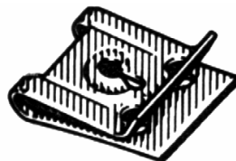
Part# 43331 #8 Screw Size Panel Range: .025" - .150" Center of Hole to Edge: 3/8" Short Unit Package: 100
