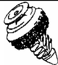
Part# 47450 Front & Rear Door Panel Retainer Hole: M9 Upper Hd: 13mm Trim Thick: 3mm O/L: 26.5mm GM Unit Package: 25
