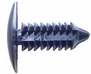
Part# 47323 7/32" Hole Size Panel Range: .110" - .460" Black Trim Panel Retainers Unit Package: 50
