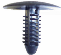
Part# 47317 9/32" Hole Size Panel Range: .100" - .510" Black Nylon Interior Trim Unit Package: 50
