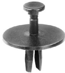
Part# 47149 Ford Luggage Compartment Trim Attachment Retainer Head 1", Stem 9/16" Fits Into 1/4" Hole Unit Package: 15
