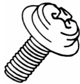
Part# 41216 License Plate Screw Phillips Pan Washer Head Dichromate Gold Finish M5-0.8 x 12mm w/12mm Washer Head Ford Contour Unit Package: 100
