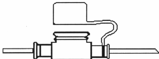
99669-MINI 30 AMP "MIBF"-TYPE WATER PROOF FUSE HOLDER 12 GAUGE WIRE
