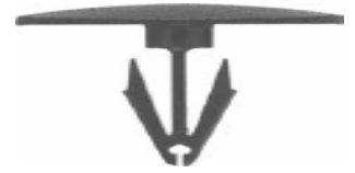
Part# 47479 Drive Type Rivet Radiator Support Sight Shield, Flange 27mm Hole M9, P.R. 9.9-11.8mm Unit Package: 15
