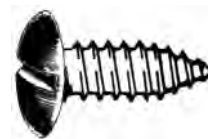
Part# 41104 Black E Coat (168 Hours Salt Spray) #14 x 3/4" License Plate Screw Slotted Truss Head 9/16" Head Diameter Unit Package: 100
