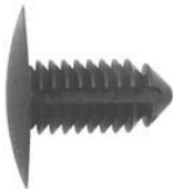
Part# 47484 Front End Retainers Black Nylon Hole 11/32" (9mm) Panel Range: 1.6 - 10mm Head: 24mm, Stem: 20mm G.M. # 22189414 25 Pcs.
