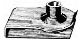
Part# 43324 Long Extruded "U" Nuts M8 - 1.25 Screw Size Panel Range: .80mm - 4.50mm Center of Hole to Edge: 20mm Unit Package: 25
