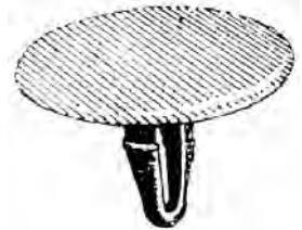
Part# 48443 Toyota Retaining Clip Head Diameter: 30mm Stem Length: 17mm Hole: 7mm, Panel: 6mm Unit Package: 25
