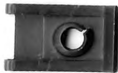
Part# 43573 Long U Nuts Black Phosphate Finish #14 Screw Size Panel Range: .025 — .150 Center: 5/8 Unit Package: 50
