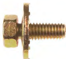
Part# 44104 M6 - 1.00 x 16mm 10mm Indented Hex Head 18.5mm O.D. Loose Washer Zinc and Yellow Finish Metric Type Body Bolts GM 11503812 Unit Package: 50
