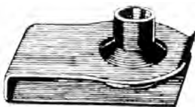
Part# 43566 "U" Nut for Pick-up Beds & Bumper Bracket M12-1.75, Throat: 42.5mm, PR 3.0-7.0 Aluminum Oxide Finish Ford Ranger, Dodge Durango Unit Package: 5
