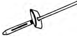
Part# 42212 Super Tough Nylon (Black) Blind Rivet Rectangular Head 8.0mm x 15.0mm Rivet Diameter: 3.96mm Grip Range 6.0 - 10.5mm Ford Unit Package: 25
