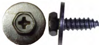
Part# 41112 M5—1.59 x 16mm Phillips Hex Head Sems 16mm Washer O.D. 8mm Hex Unit Package: 50
