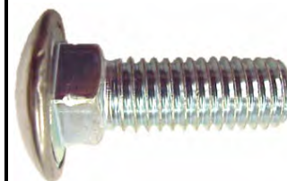
Part# 44350 7/16-14 x 1-1/2" 15/16" Head Diameter Round Head Style Stainless Steel Capped Bumper Bolts Unit Package: 25
