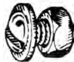
Part# 41107 1/4" -20 x 9/16" Zinc Slotted Round Washer Head License Plate Screw with Hex Nut 9/16" Washer Head O.D. 7/16" Hex Width (ATF) Unit Package: 100 Sets
