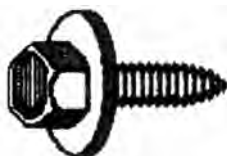
Part# 44347 M6 - 1.00 x 20mm 10mm Indented Hex Head 17mm O.D. Loose Washer Black Phosphate Finish Metric Type CA Body Bolts Unit Package: 50
