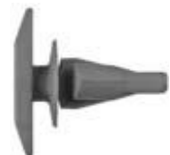
Part# 47487 Weatherstrip Retainers Blue Nylon Hole 13/64" Head 5mm x 14mm Stem 10mm Ford Unit Package: 100
