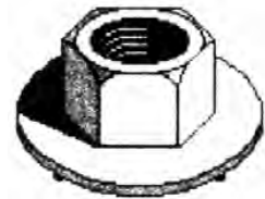
Part# 43210 8-1.25mm Metric Hex Nuts 13mm Hex Size 24mm O.D. Loose Barbed Washer Black Phosphate Finish Unit Package: 25
