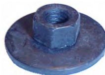
Part# 43567 Not supplied by OEM Nut with Free Spinning Washer M6-1.0 with 24mm Loose Washer 10mm A/F, Grade 9 Black Finish, General Purpose Unit Package: 50
