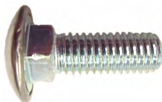
Part# 44348 1/2-13 x 1-1/2" 1-3/32" Head Diameter Round Head Style Stainless Steel Capped Bumper Bolts Unit Package: 25
