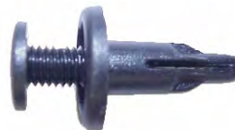
Part# 48459 Plastic Drive Rivet Head: 18mm Stem: 21mm Grip: 4—8mm Hole: 8mm Unit Package: 10
