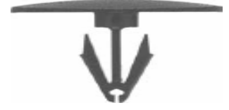
Part# 47473 Rocker Panel Molding Clip Black Nylon, Hole 5/16 Head Dia 11/16 x 1-5/16 GM 10431524 Unit Package: 15
