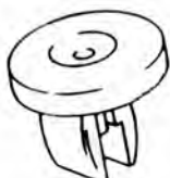
Part# 47255 Plastic Nut Grommet 20mm Face Screw Size 4.8mm Hole: 11.5 x 8.2mm Cowl & Various Trim Panels Ford Unit Package: 25
