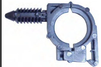
Part# 47164 Wire Loom Routing Clip For 1/2" ID, 11/16" OD Loom Stem Diameter: 3/8" x 2-1/2" Stem Length: 1/2" Fits Into 1/4" Hole Unit Package: 15
