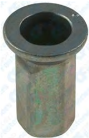
Part# 43575 Specialty Nutsert Zinc & Yellow Thread Size: M6-1.0 Grip: .65mm - 2.0mm Head Diameter: 12mm Hex Size: 8mm GM: 15685099 Ford: N803763-S100 Unit Package: 15
