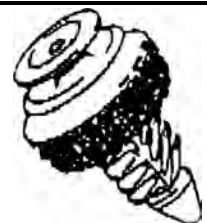
Part# 47450 Front & Rear Door Panel Retainer Hole: M9 Upper Hd: 13mm Trim Thick: 3mm O/L: 26.5mm GM Unit Package: 25
