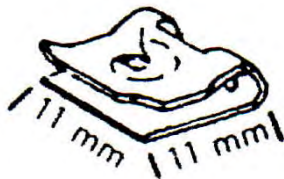
Part# 43224 Replaces U Type M4.2 - 1.41 Panel Range: 1.47 - 2.30mm Back/Center 7.0mm Black Finish Unit Package: 100
