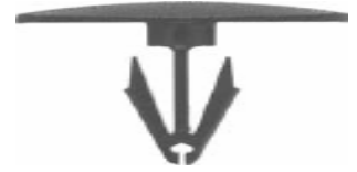
Part# 47479 Drive Type Rivet Radiator Support Sight Shield, Flange 27mm Hole M9, P.R. 9.9-11.8mm Unit Package: 15
