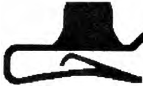
Part# 43340 Extruded "U" Nuts 10 - 1.50mm Panel Range: .035" - .232" Center of Hole to Edge: 3/4" Black Phosphate Finish Unit Package: 25
