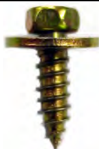
Part# 41111 Zinc & Yellow Dichromate M5.5-1.81 x 18mm #12 x 45/64" 15mm Washer, 8mm Hex Unit Package: 50
